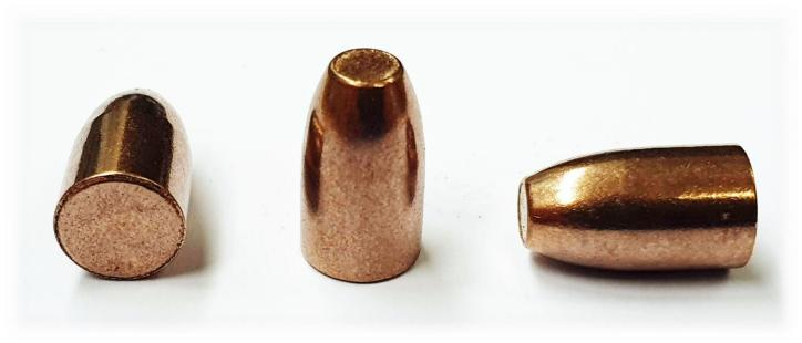
The 9x19mm Frangible projectile was designed as a sustainable alternative to normal Full Metal Jacket projectiles with lead core. It is completely lead free and manufactured by sintering of a customized metal powder mix. It has frangible properties, *i.e.*, fragmenting when hitting hard targets like steel plates and poppers, making it very suitable for all kinds of training and competition, especially at indoor shooting ranges, where lead is a health hazard.
